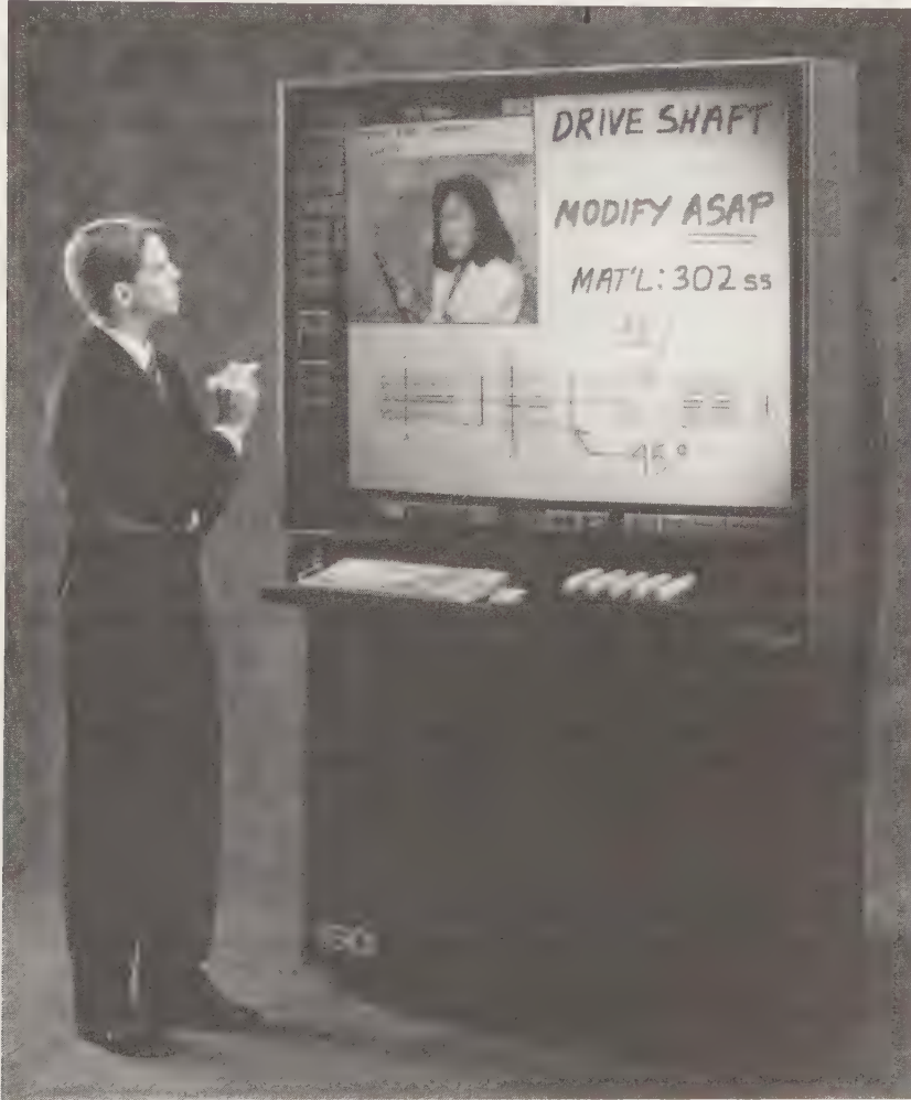
Figure 2.1 The product version of the Xerox Liveboard. The Liveboard has keyboard, mouse and pens for input. Tivoli is shown on the display, with the soft control buttons on the left and bottom of the display. A video window overlays the Tivoli window. The Tivoli page has an important image which is being annotated with Tivoli strokes.
